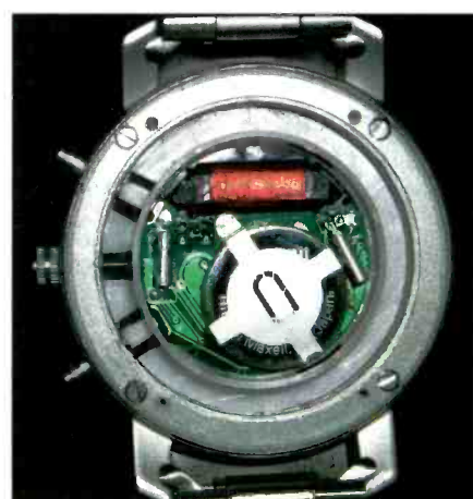
The interior of a low cost watch controlled by WWVB signals. Note the ferrite bar antenna and two crystal oscillators, one a 32.768 kHz crystal that drives the quartz clock, the other is a 60 kHz crystal that serves as a pre-selector for the time signal. The battery appears to take up more area than the crystals and antenna combined.
