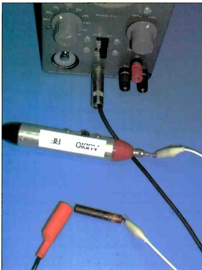
Photo F. Here's the noise switch feature being used to test a suspect carbon resistor.
