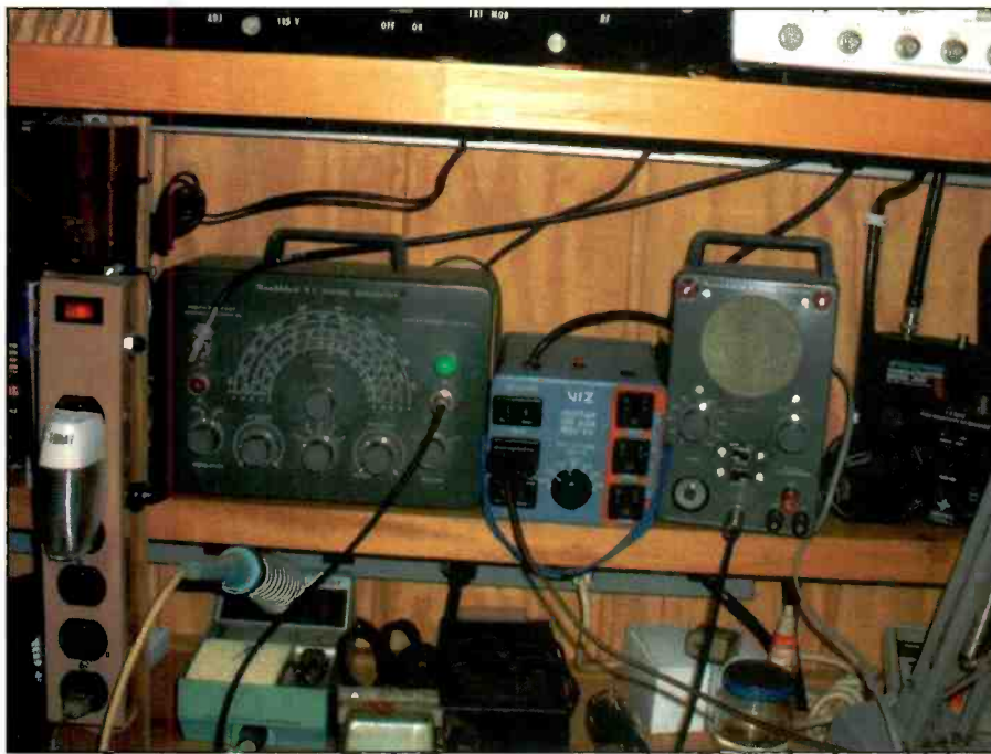
Photo B. Here's an example of a test bench being used to signal trace a problem in an old radio. The test gear includes the signal tracer, a signal generator, and an AC line isolation transformer. The isolation transformer should always be used to power the radio, regardless of whether the set is an AC/DC type with a hot chassis or a transformer-operated design.
