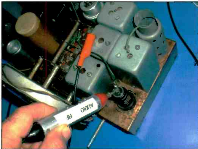
Photo D. The tube grid caps often provide very convenient monitoring points for the signal tracer!
