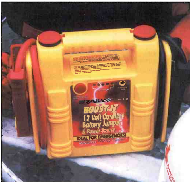
This small "minimum" battery is adequate for short periods of time.
