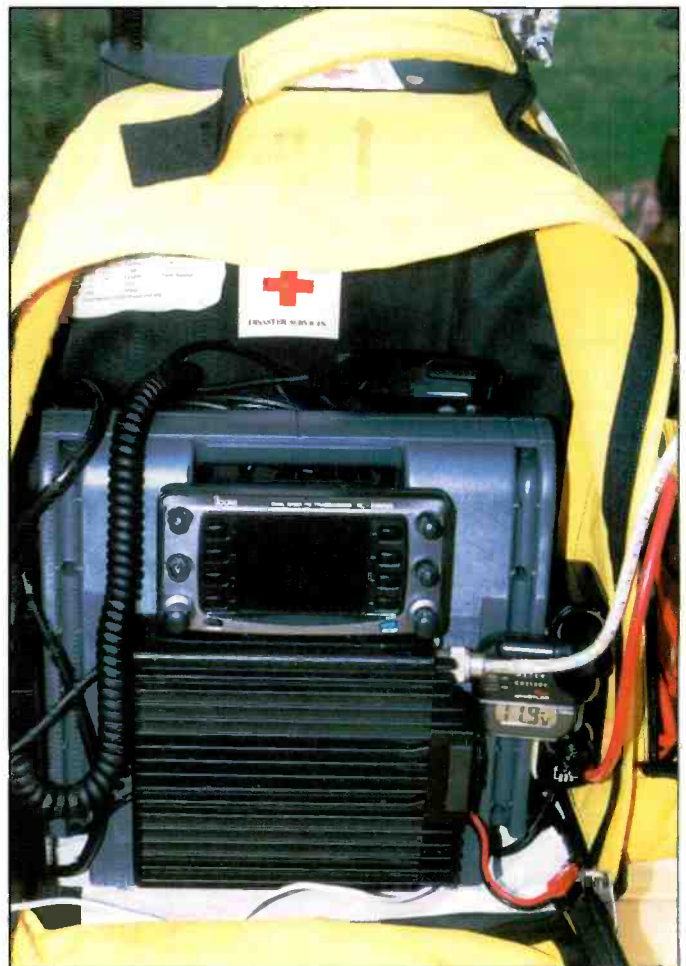
Here's a major-size 17-amp-hour battery system with a mobile VHF/UHF radio attached.
