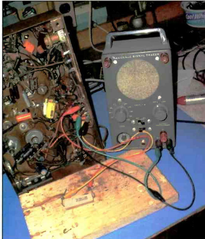
Photo E. Subbing the Zenith speaker, transformer, and field coil.
