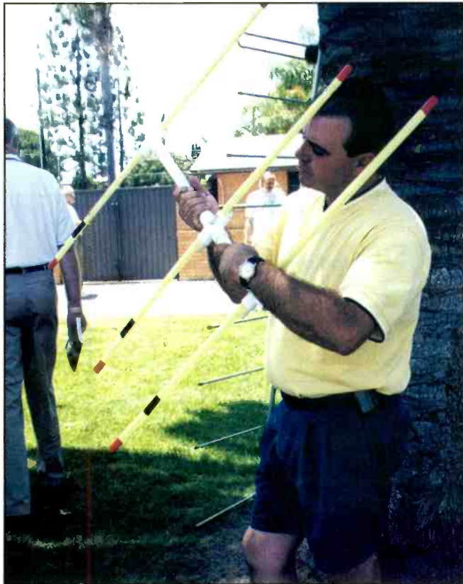
A small homebrew MURS 153-MHz beam extends range and can cut down on interference.
