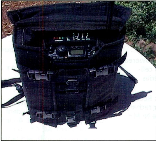
Here is an FT-817/LDG Z-11 tuner combo in a Communications Outfitters pack complete with onboard HF antenna. This system can be carried with little effort and used as pedestrian mobile from almost anywhere.
