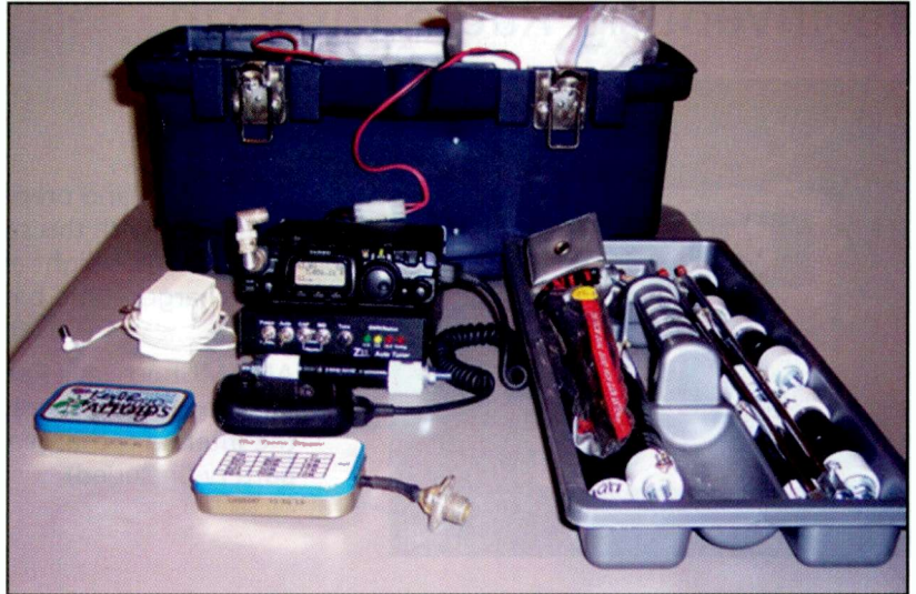
Another version of a jump kit centering on the ultra versatile FT-817/LDG Z-11 tuner. This kit features a PAC-12 HF multiband dipole antenna, antenna alignment device, and internal battery and charger, all built into a tool box available from many home improvement stores. This is a very rugged jump kit that is ready to go on short notice.
