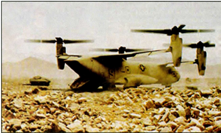
The "Quad" Tilt rotor concept being studied by the Pentagon, a C-130 sized troop/cargo transport based on V-22 technology.
