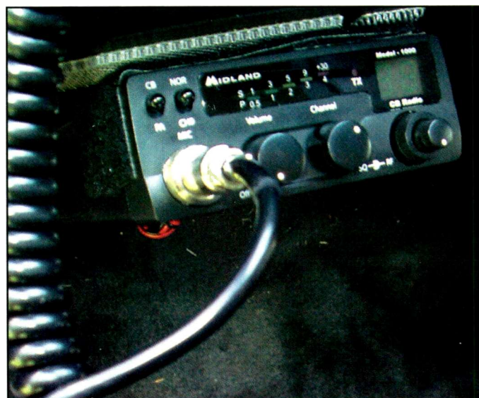
Mounted and ready to hit the road, the Midland 1001Z fits perfectly and is light enough to use heavy-duty hook-and-loop fastener.
