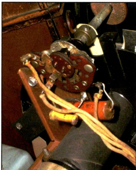
Photo A. The tone control wafer switch on a 1938 model Zenith Shutter Dial chassis can be damaged if the chassis is laid upside down on a workbench without proper support.
