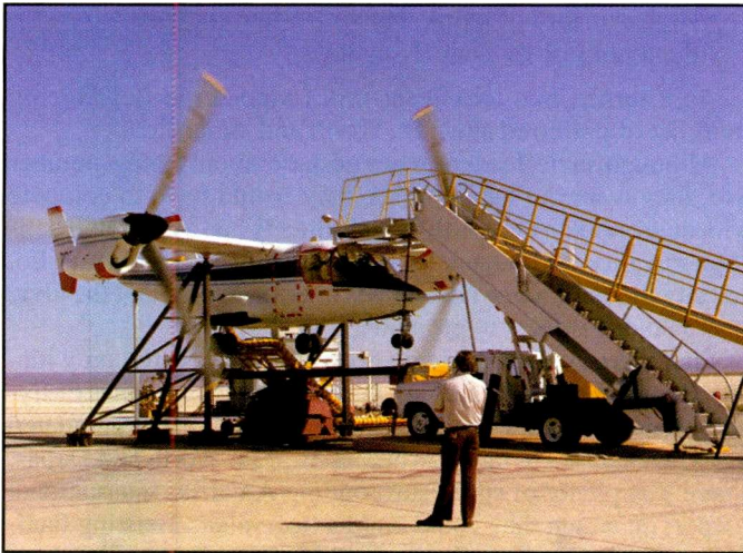
A XV-15 on a test stand at Edwards Air Force Base. (Photo courtesy NASA/Dryden Flight Research Center Archives)
