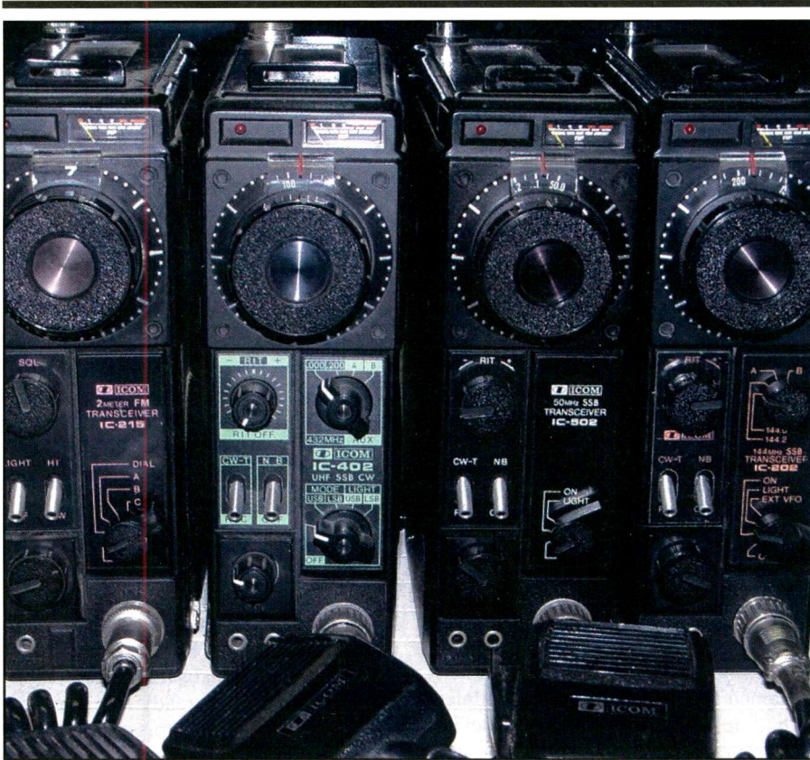
Here's the complete set of ICOM "Bookcase" radios circa 1979-1984. All these little rigs seemed to be a bigger hit in Europe than here in the States. The three SSB/CW radios, the IC-402, 502, and 202 (from left, the second through fourth in the picture) are 3-watt PEP output on SSB and about 1.5-watt output on CW. The IC-215, the left-most radio, is a 1- to 10-watt, 2-meter FM transceiver that uses crystals and has 15 channels. This set was assembled for under $300 by watching eBay and eHam.net and pouncing on bargains. These rigs are going to Field Day with me to provide the VHF/UHF station.
