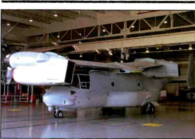
MV-22s fold up for compact storage on aircraft carrier decks. Note the mangled propeller on this Osprey. (Photo by Steve Douglass)
