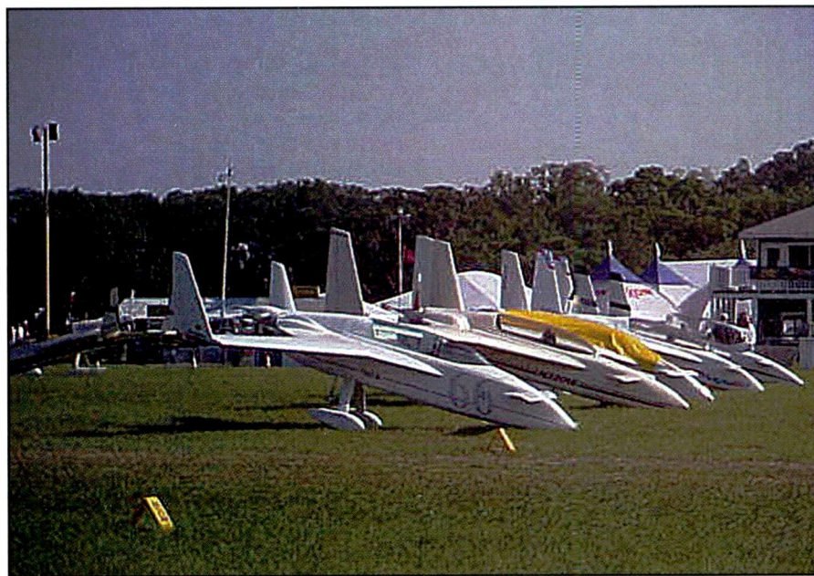
On the flight line, these odd looking aircraft with the noses on the ground are Rutan Vari-E-Zs. They are one of the most popular homebuilt aircraft, most seating one or two and with cruise speeds for some reaching into the high 100s/low 200s.
