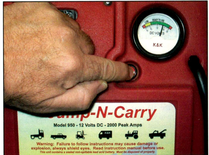
Push the button for a quick meter reading that gives you an instant status of the unit's battery power.
