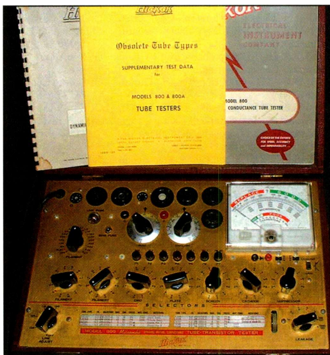
Photo A. The Hickok 800 is a versatile and popular tube tester. It can test a majority of the tube types used in early radios. The Hickok obsolete tube data booklet accompanied this tester; it shows how to set up the device to test early obsolete tube types.
