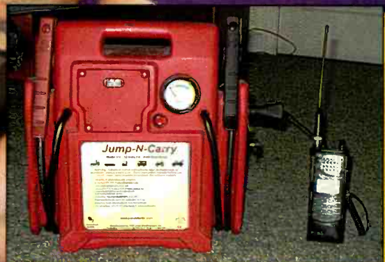
Tech Showcase: Clore Automotive's Jump-N-Carry power supply with an Alinco DJ-G5T transceiver. Pg. 16.
