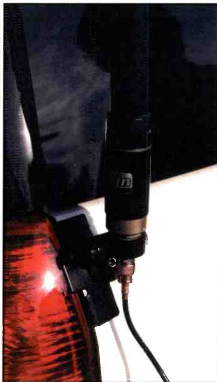
A trunk-lip mount on the SUV will hold some very tall antenna systems.
