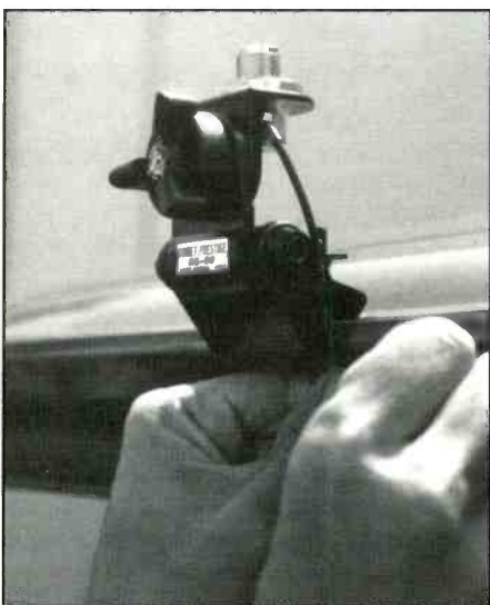
The small RG-188 coax goes under the vehicle's door jamb, then changes to large RG-9913 type coax.
