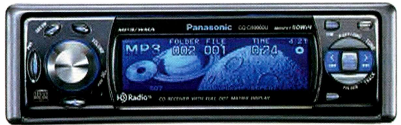
Panasonic's CQ-CB9900U receiver includes a CD player, dot matrix graphic display, and DSP for improved sound quality.
