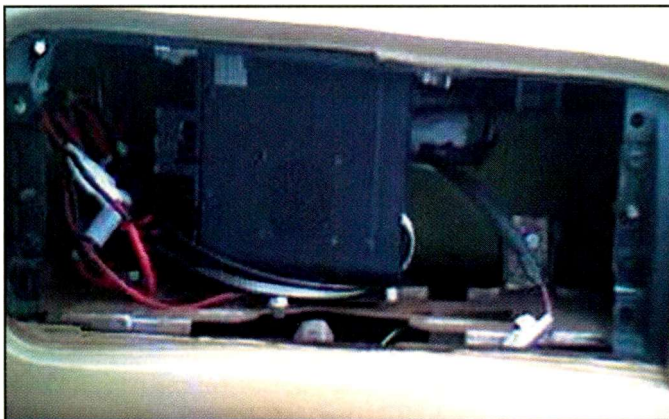
Scott, KD5PCK, shows us his mobile transceiver installation, located behind a dummy airbag panel. (Photo courtesy of KD5PCK)
