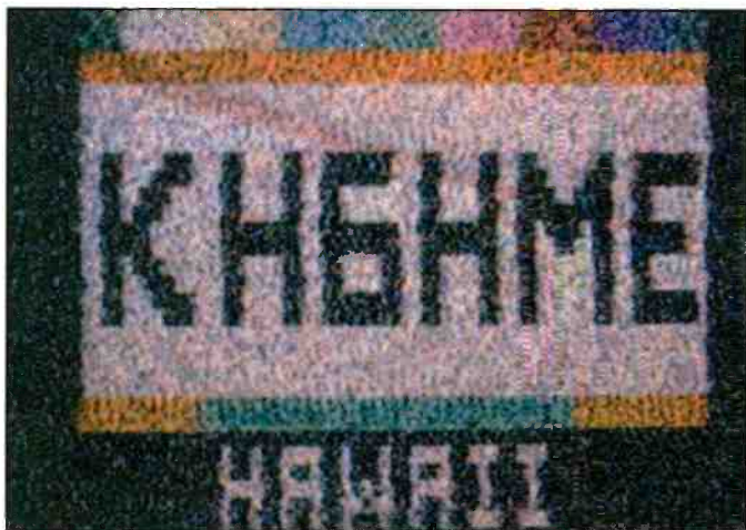
Here’s a look at the first-ever Amateur TV reception of the Hawaii 426-MHz beacon in California at Gordo’s station. Reception was due to tropo ducting.
