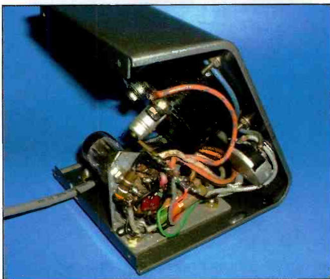
Photo D. Most of the component leads are supported between the solder terminal strip and the 9-pin 12AU7 tube socket. Vintage parts were used when available. Insulated tubing covers bare component leads for neatness and to minimize the chance of shorts.
