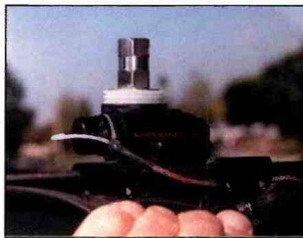
Four Allen screws hold this lip mount securely to the top of the rear door.
