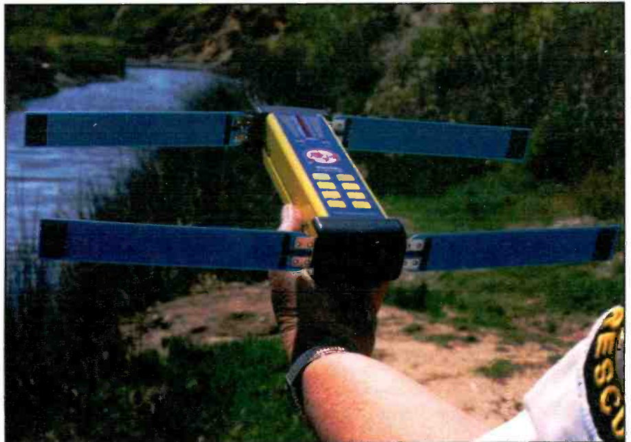
The ACR direction finder in a real 121.5 MHz track-down along a popular river's remote rafting area.
