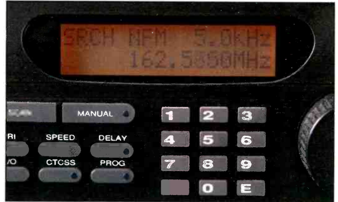
Searching is much easier on newer receivers than it used to be. Just make sure you set an upper and lower limit that are not too far apart.
