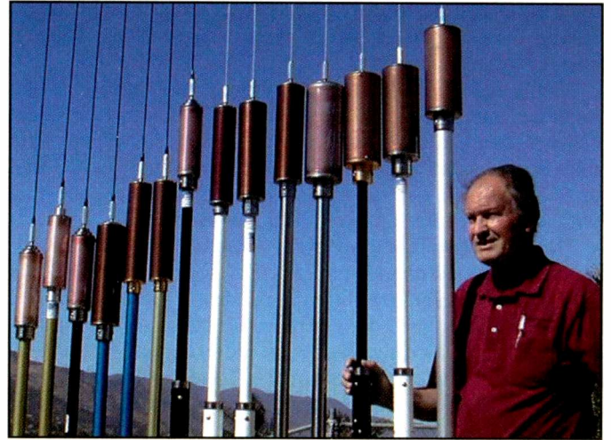
Here's Charlie Gyenes, W6HIQ, of Wildomar, California, who manufactures a large line of high-quality, high-performance mobile antennas. These are mostly motorized, center-loaded whips suitable for use on cars, boats, or even balcony railings. Check out the entire line at the Hi-Q-Antennas website, www.hiqantennas.com . They're so "purdy" it's almost a shame to mount them on the back of the car!
