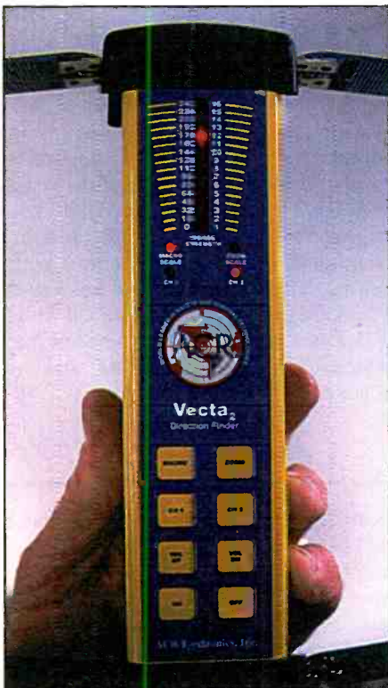
The ACR direction finder with red LEDs which travel from bottom to top when headed toward the station
