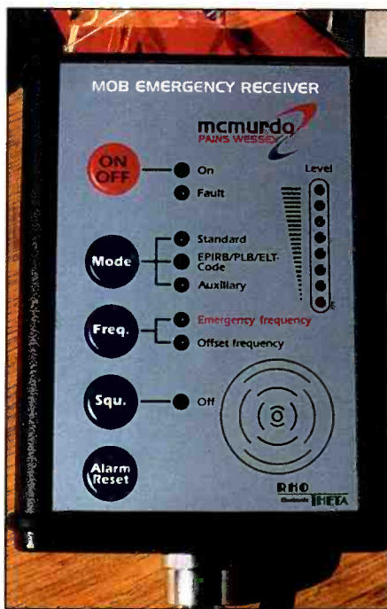
The local harbor patrol has this 121.5 MHz receiver mounted and turned on ready for an emergency alert!
