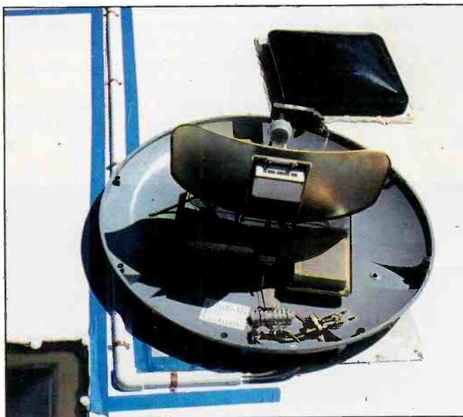
Most motorhomes have a vent area that comes up behind the refrigerator. By removing the vent cap you can run the wires down the back of the refrigerator vent area to where you are going to have your satellite receiver mounted. Art used 3/4-inch PVC pipe cut halfway down the middle to cover the wires.
