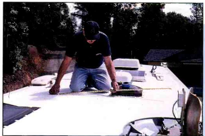
Carefully tape measure for center roof line.
