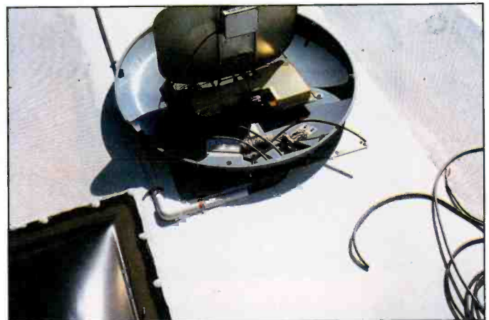
After cleaning the base plate of all debris, you can now install the antenna unit back onto the base plate.
