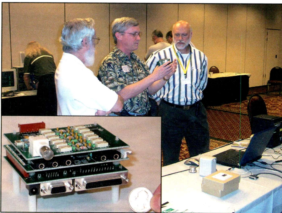
Gerald Youngblood, AC5OG, discusses the SDR-1000 Software Defined Radio with Ron Block, KB2UYT (left), and Phil Thies, K3TUF (right), at last September's ARRL/TAPR Digital Communications Conference in Connecticut. Inset is the SDR-1000 semi-kit board set. The SDR-1000 is a Software Defined Radio, where all signal processing is performed in software, using a PC sound card. It's much more than a software-controlled or DSP radio (see text for more info).
