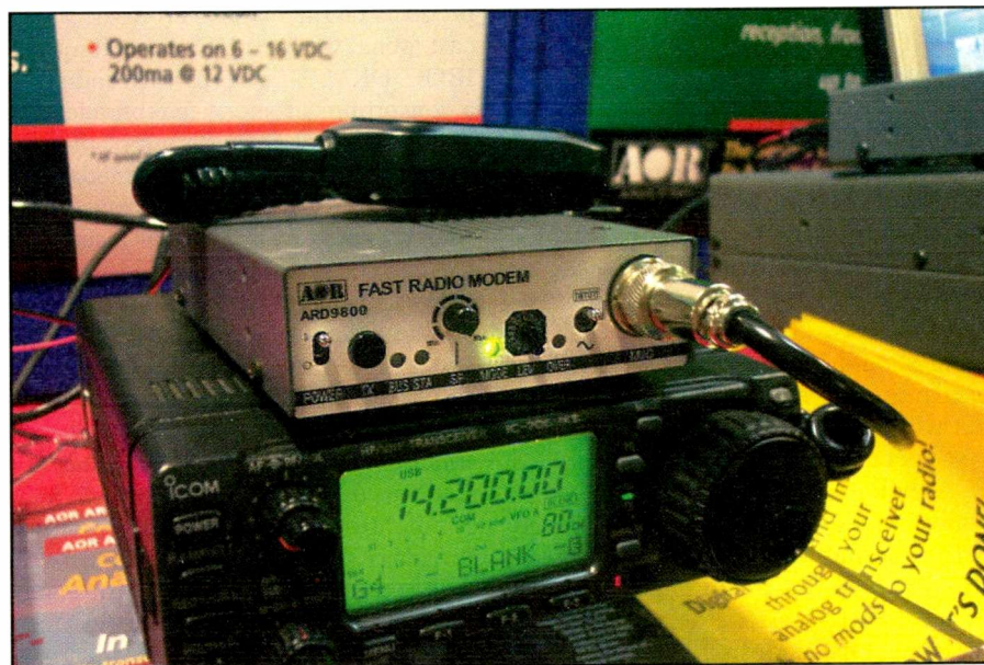
The AOR ADR8200 digital voice “adapter,” sitting atop a typical HF transceiver. This little box takes your voice and turns it into a digital voice signal that can be transmitted through almost any radio. You’ll need another one at the receiving end to hear what’s being said, however. Although the technology involved is a steal at $500, casual listeners will probably continue to wait for less expensive solutions.
