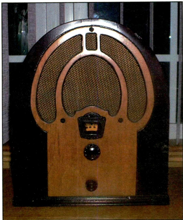
Photo A. This small Philco cathedral uses four tubes and a regenerative IF to improve gain.
