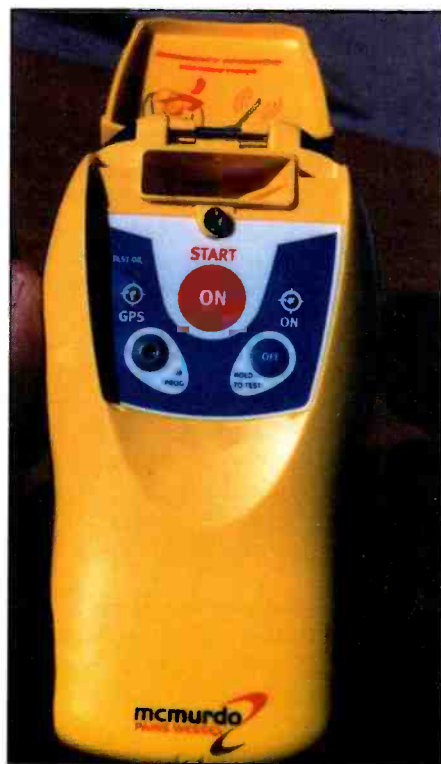
This 121.5 MHz also transmits 406.028 MHz position reports with a built-in GPS.
