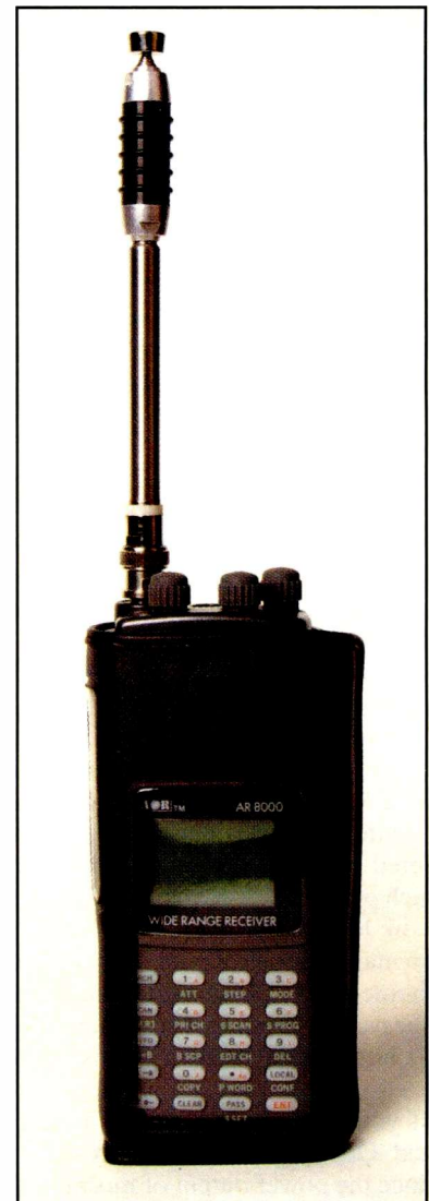
This telescopic whip from RadioShack has been an old standby for many years. A broadband receiver needs an antenna that can adjust to a wide range of frequencies.
