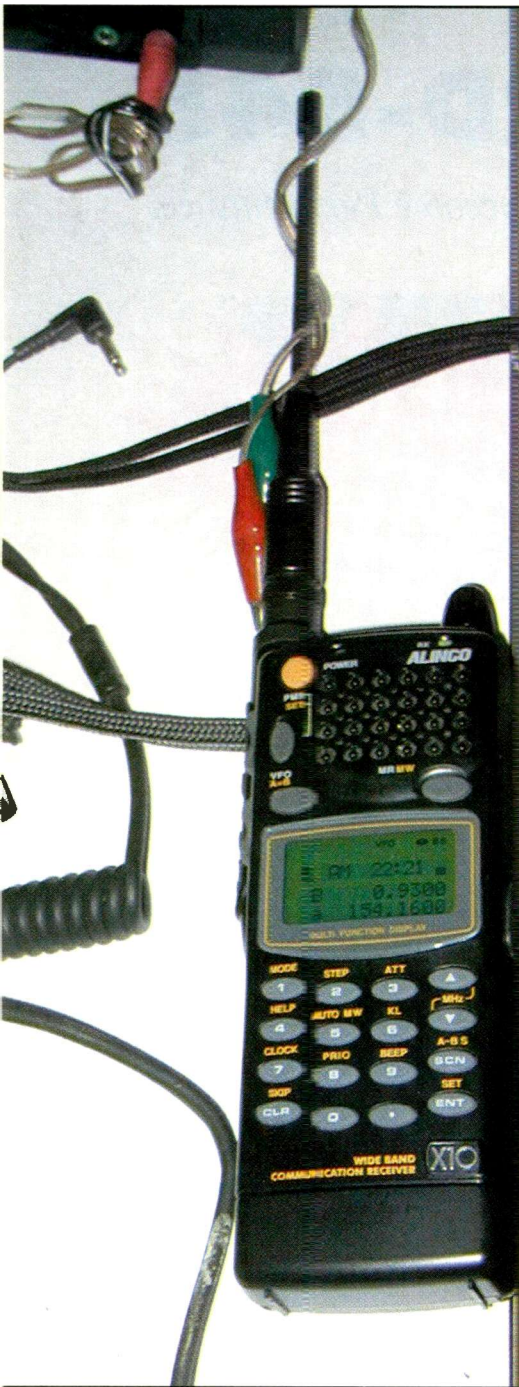
AM inductive coupling to a long wire nets a better signal.
