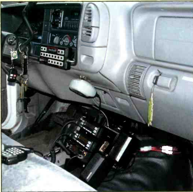
The "radio stack" in the front of the Mobile Command Post is composed of (top to bottom) Kenwood UHF and VHF Public Safety transceivers sitting on top of a Kenwood 2-meter transceiver. The siren/lightbar controls are above and to the left (on the dashboard). From this position the driver can access some of the capabilities of this communications vehicle while in motion.
