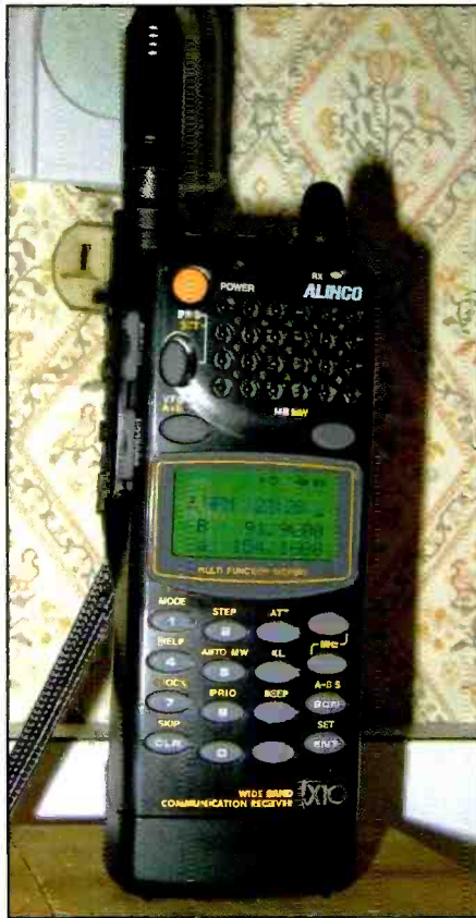
An FM broadcast test using capacitive coupling to AC wiring yields a better signal than the rubber duck.
