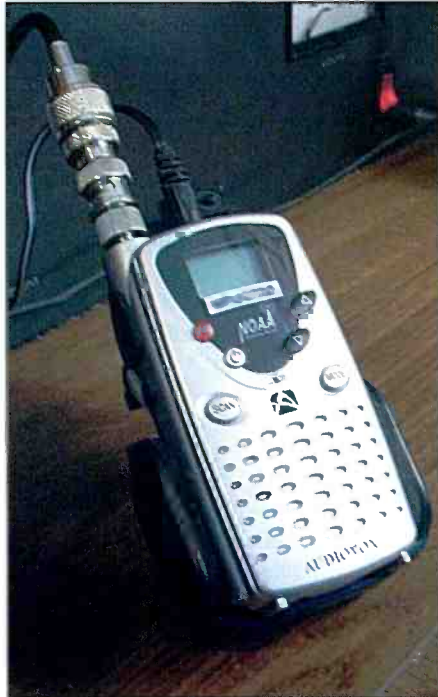
Photo C. Our GMRS bubble-pack handheld, mounted and connected to antenna and power supply leads for base station use.
