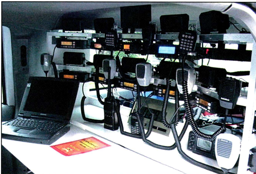
The operating position from the driver's side shows a slightly better angle on the gear. While this might look perplexing, once the operator has a short tutorial this is an easy station to operate. The laptop is used for digital modes as well as to program the radios while in the field. Note the two small handhelds: a VHF EMS radio, and an ICOM air-band transceiver for contacting airborne Life Flight/Life Lion medevac choppers.
