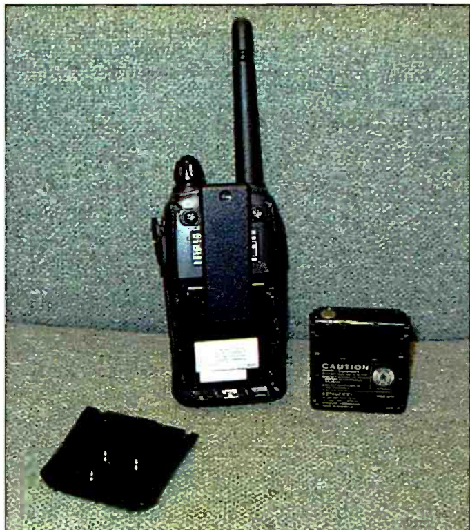
This NiCd battery pack from a RadioShack HTX-202 amateur transceiver will lose about 30 percent of its charge in a month.
