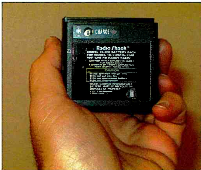
This NiCd battery pack from a RadioShack HTX-202 amateur transceiver will lose about 30 percent of its charge in a month.
