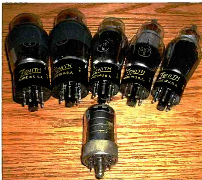
Photo D. These Zenith ST-shaped tubes are typical of what was supplied with circa-1940 Zenith consoles. It's a thrill finding the original Zenith tube set in a radio! The 7G7 RF amplifier tube in front is an example of a Loctal base tube.
