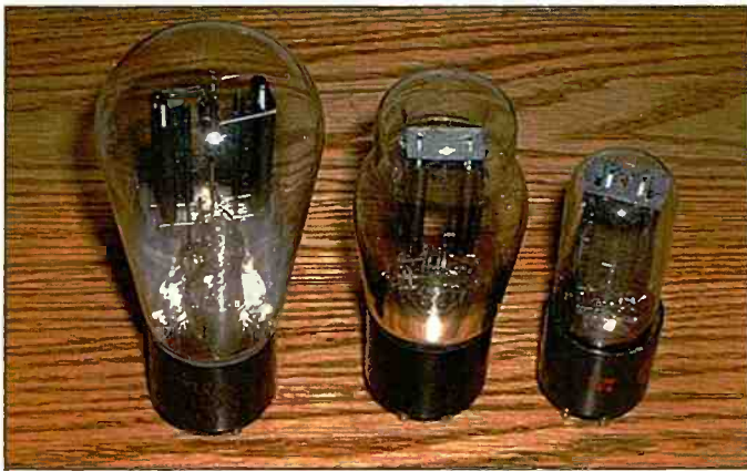
Photo C. Arguably, few tubes can boast having as long a production as was enjoyed by the 80 full-wave rectifier. Here are three examples spanning the decades. The globe-shaped early 80 was introduced in the late 1920s, the ST-shaped in the late '30s, and the tubular version continued until production ceased. The "modern" electrical equivalent for the 4-pin 80 would be a 5Y3G(T) octal.
