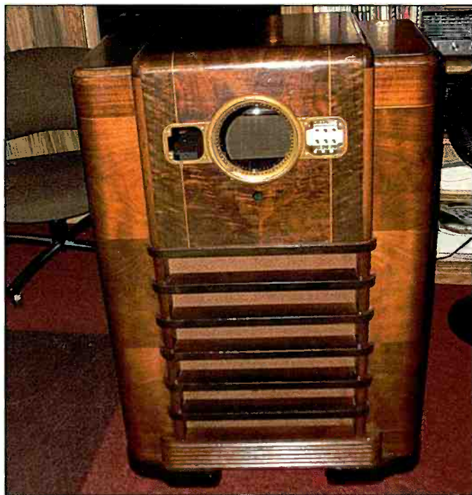
Photo A. The refinished 10S464 cabinet with a hand-rubbed piano finish. The replacement grille cloth came from John Okolowicz's Grille Cloth Headquarters. (See Reference 2.)
