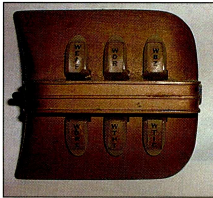
Photo F. The "ironing board" key assembly for the station presets was missing. A replacement was made by modifying a tone control panel for the 1005 Zenith chassis. This part was purchased from Joann Frush. (See Reference 2.)
