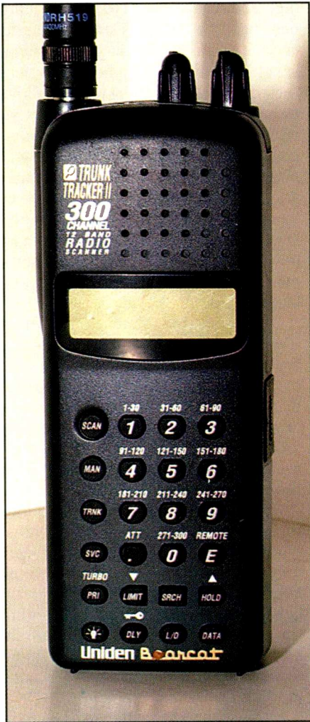
This Uniden BC245 trunktracker is probably one of the most capable trunktrackers on the market and it's relatively easy to use (once you get used to it). Learning to program any trunking radio can be a challenge!
