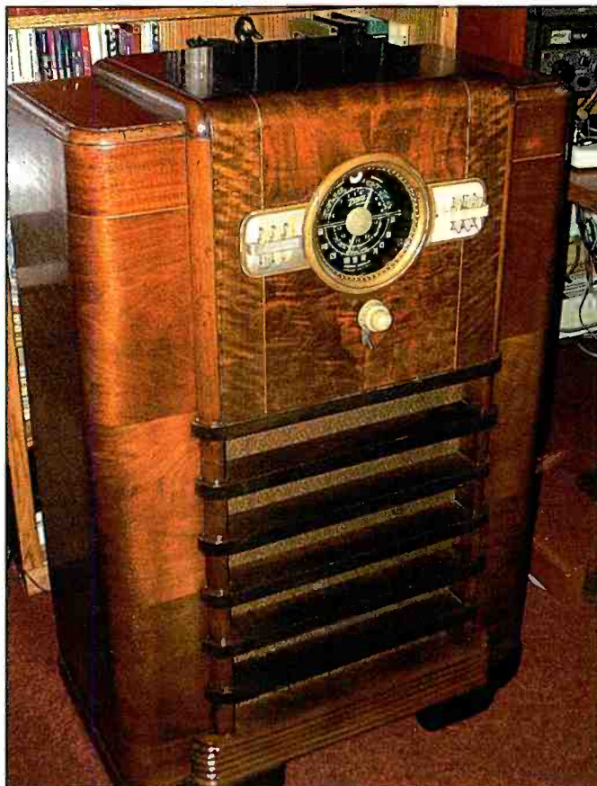
Photo B. The 10S464 after restoration. The radio was run for a few weeks to burn it in and to make sure no problems would surface after it was returned to its owners.
