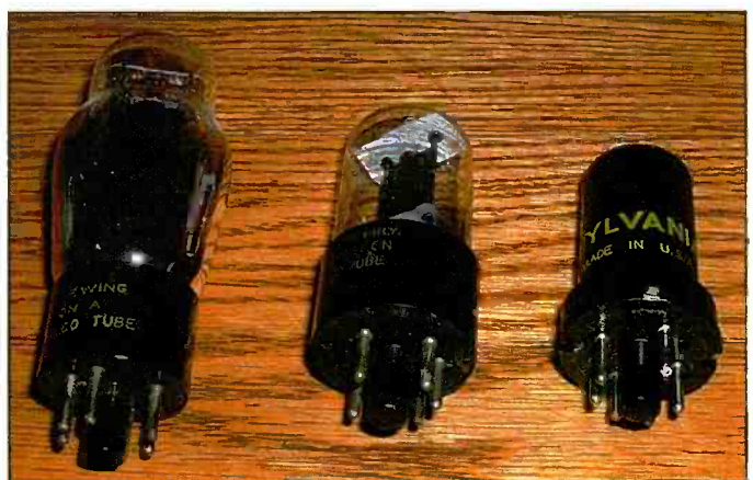
Photo E. Three versions of the 6J5 triode are shown here: ST (or shouldered glass), tubular, and a metal Sylvania brand 6J5 tube.
