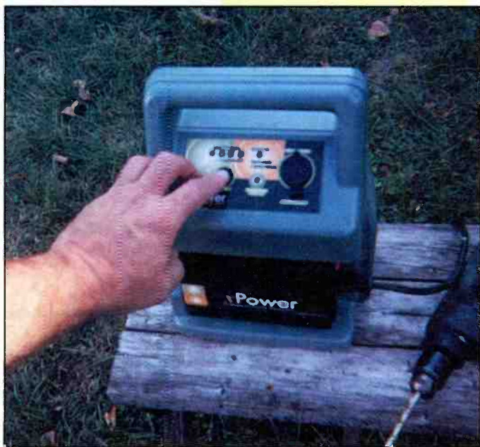
Push the button for an instant look at the xPower 300's battery condition.
