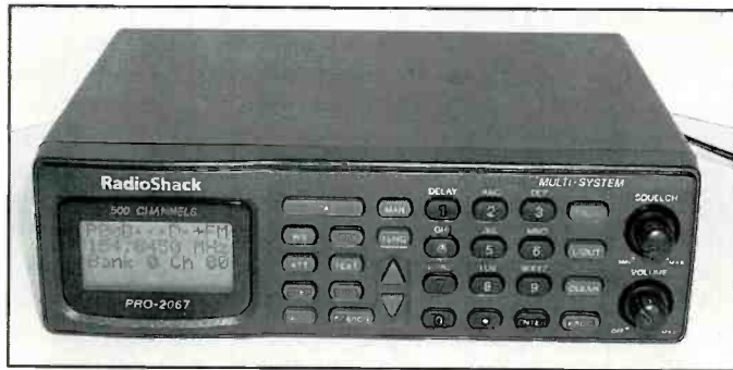
The PRO-2067 from RadioShack is a base or mobile scanner with trunktracking capabilities, and can display the channel you're listening to with alphanumeric characters instead of a channel number and frequency!
