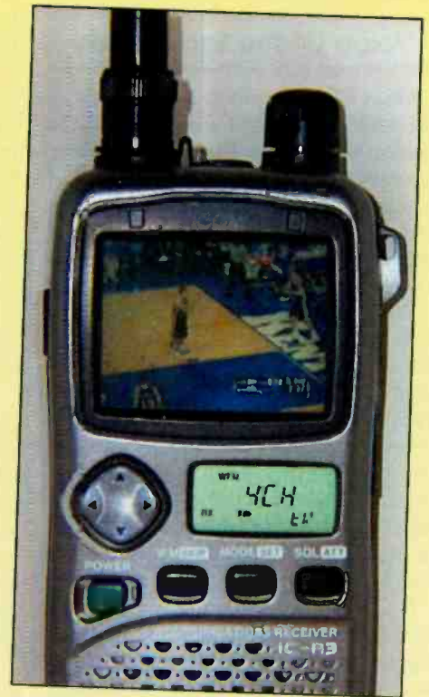
The R3 in TV mode. Note the smaller LCD display showing the TV mode and Channel 4 (That's KMOV, here in St. Louis). The smaller LCD can be used in all modes to show limited information and preserve battery life. You can even listen to TV audio with no picture if you prefer.
