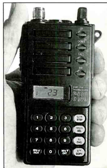
The Pryme portable programmer looks like a Standard Radio Corp. transceiver, but it is not a radio!
