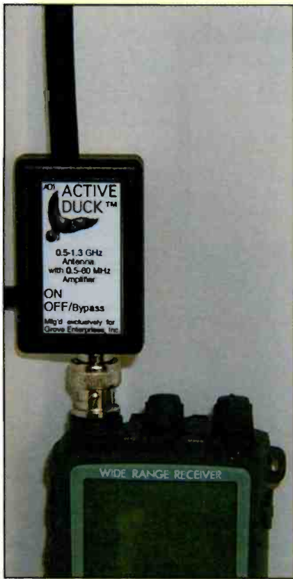
This active but portable antenna is ideal for wideband receivers such as the AOR-AR8200 if you want to listen to HF and VHF low frequencies up to about 60 MHz.
