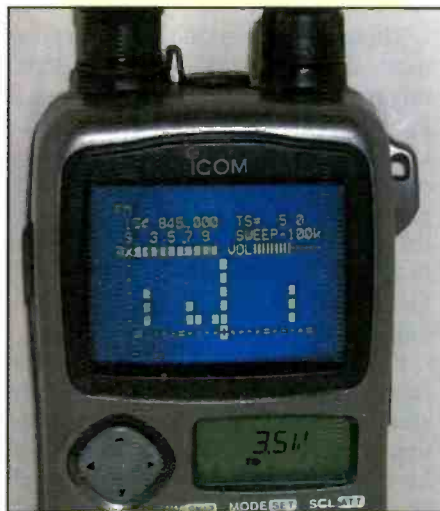
Here's the handscope display showing activity on a few neighboring channels.
