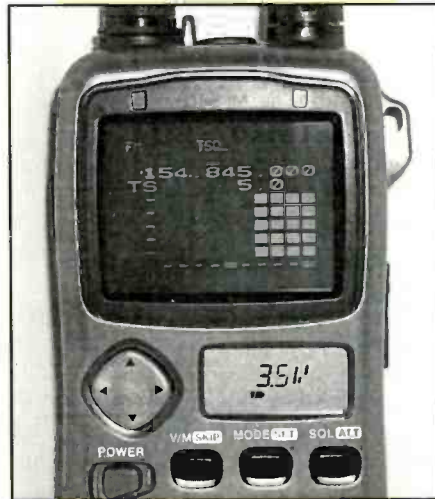
The final mode is the signal strength vs. time plot. Here, a strong station was transmitting and then stopped, so it's strong signal strength bars are scrolling off to the right.
