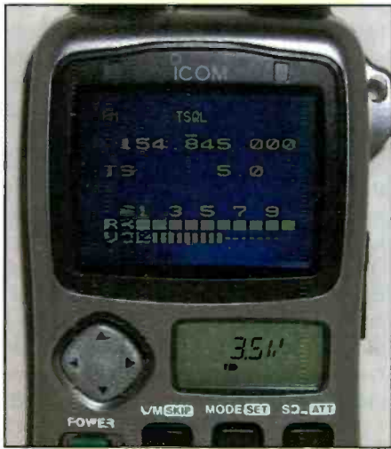
Here's the full data screen display showing frequency, signal strength, volume, and other settings. It's easy to read!
