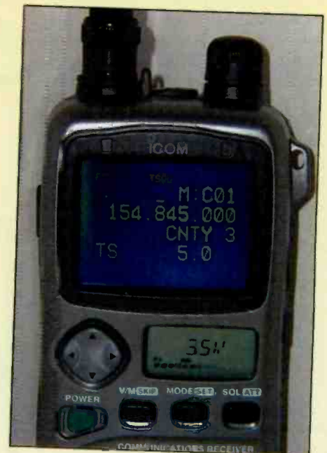
The memory display includes the alpha tag display, but unfortunately the battery life is reduced with the LCD turned on.
