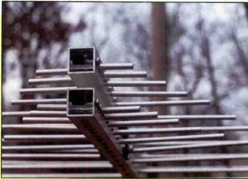
The coax is fed to two stainless steel sheet metal screws at the end of each boom.
