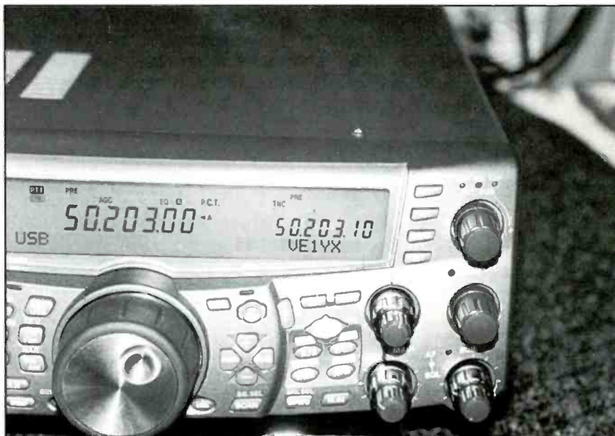
Close-up of the TS-2000's LCD panel showing active packetcluster frequency capture, plus call sign.
