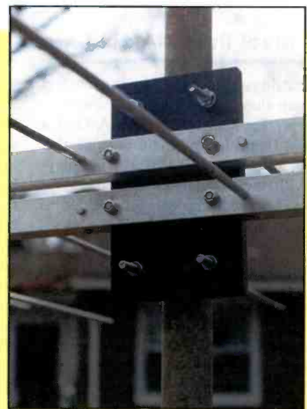
The antenna's substantial mast-to-boom insulator is also made from PVC. All hardware is stainless steel.
