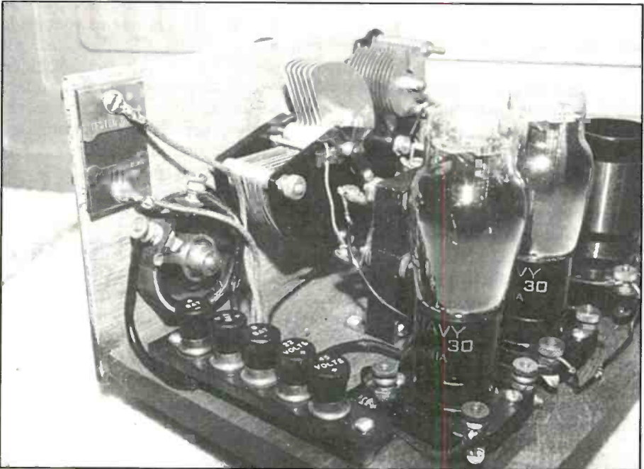
The silvery inside of these two type 30 tubes, shown in this photo of our Boy's First Receiver project, resulted from the getters being fired after the vacuum was applied during the tubes' manufacture. This action burned off any residual gases remaining inside the tubes.
