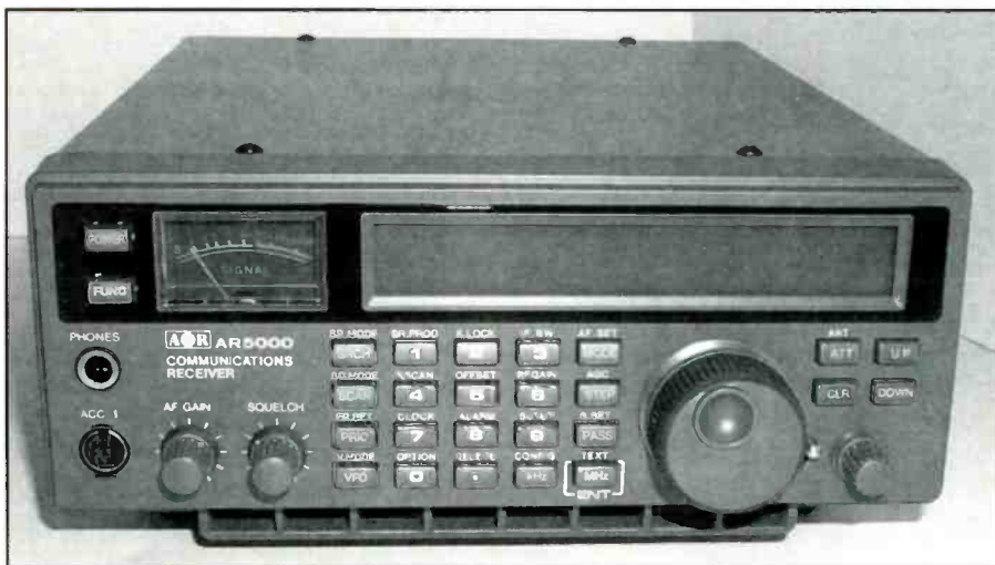
Wideband high performance receivers like this AR-5000 and many others are a wonderful addition to your shack, but don't expect too much from scanning the whole spectrum at once!
