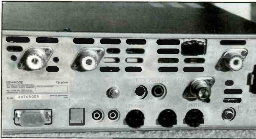
The rear panel has four antenna jacks, plus one additional spot for 1.2 GHz.
