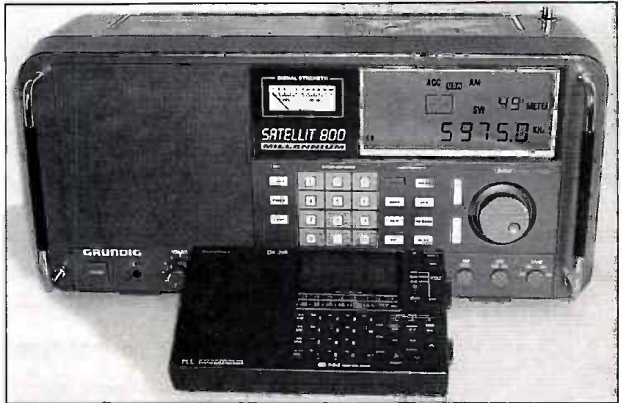
It's BIG. That's a RadioShack DX-398 sitting in front of it, which is not exactly a small portable!
