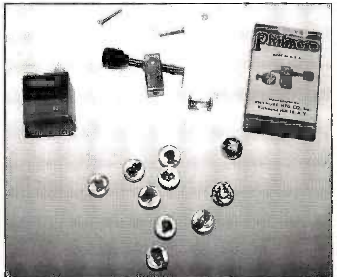
More Philmore crystal set components. At left is a box for the Philmore model 7004 mounted galena crystals. Several 7004 galena crystals, mounted in Wood's Metal, are shown. At center is a Philmore model 7010 unmounted crystal detector stand. This is very similar to the model 310 shown in top photo, but it did not include a mounting board. A builder would most likely assemble this detector on a bakelite front panel. (From the author's collection.)
