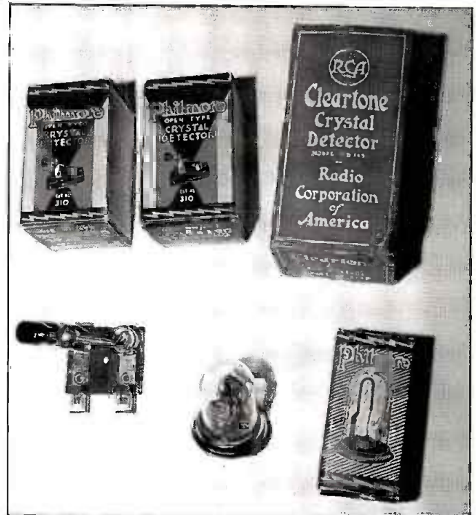
Two boxes housing mounted Philmore model 310 adjustable detectors. One of the model 310 stands is shown just below the two Philmore boxes. At top right is a box for an RCA Cleartone crystal Detector. Although the box is empty, the vintage container itself has collector value as a display item. At lower right is a Philmore model 309. Although it was sold as a fixed detector, the glass dome could be removed allowing adjustment to the cat's whisker, or replacement of the galena crystal. This Philmore 309 also is shown with its original box which greatly adds to the value. New-In-Box (NIB) vintage detectors are very collectable. (From the author's collection.)
