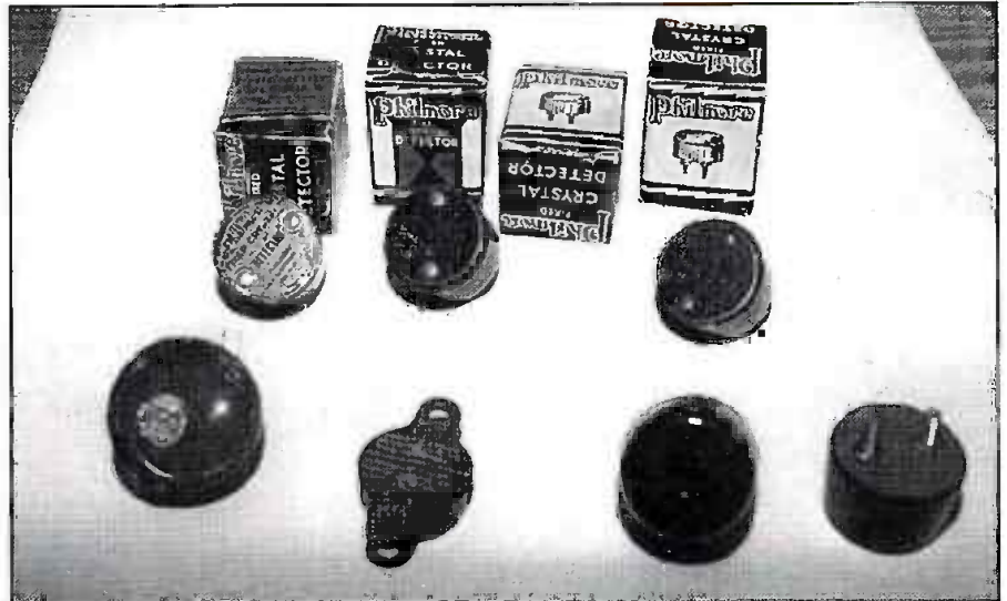
Along the top are four boxes for Philmore model 7002 fixed detectors. Just below the boxes are three of the cylinder-shaped 7002 detectors. At lower left is a fixed detector by an unknown manufacturer — a clear cover protects the cats whisker and galena crystal. The device with two mounting ears, second from the left, is an early Erla fixed detector. At bottom right are two views of another style of fixed detector from an unknown manufacturer. A small peephole allows viewing of the setting, and I assume some limited adjustment. (From the author's collection.)
