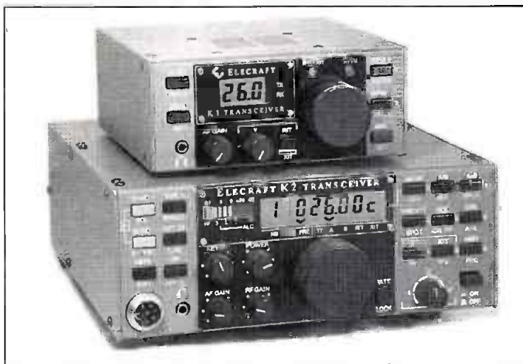
Without a doubt, the Elecraft K2 (K1 is on top) multimode, multiband HF transceiver is the pick of the litter when it comes to modern kit-built radios. The little K2 offers commercial-grade performance in a compact package that doesn't take a rocket scientist to successfully assemble and use. Do-it-yourselfers are raving about Elecraft's K-series radios. Get all the details at www.elecraft.com .
