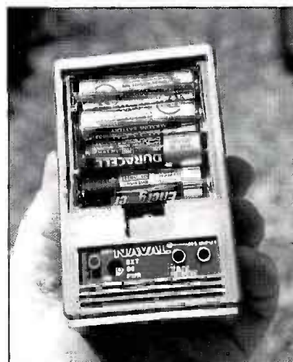
Built-in battery compartment for the Naval Electronics speaker system.
