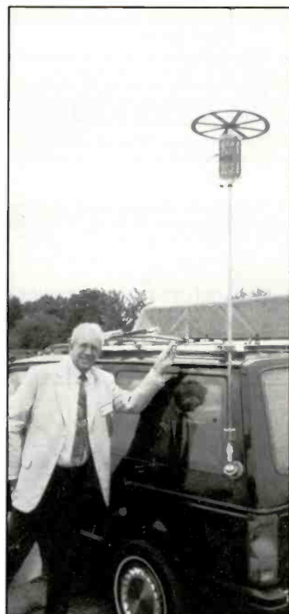
Gordon West shows off top-loading capacity hats for big signal results.
