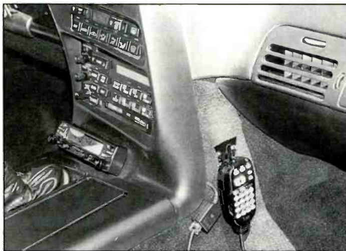
A remote head mounted too low (left) and one on top of dash near a GPS unit.
