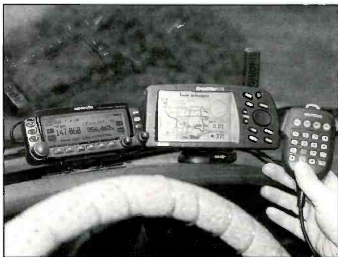
A remote head mounted too low (left) and one on top of dash near a GPS unit.
