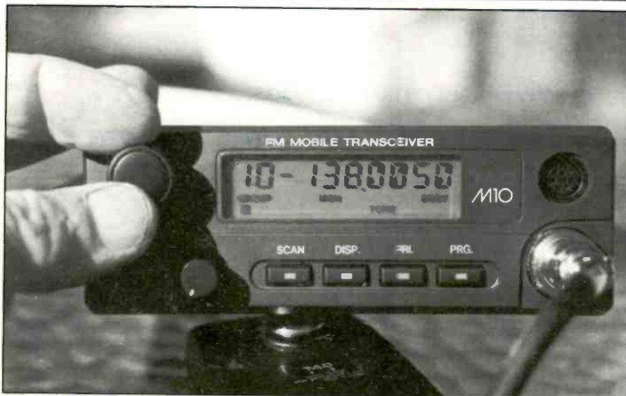
The TAD M-10 is computer programmable and offers a very tight receiver. Note the input port at the right for programming.
