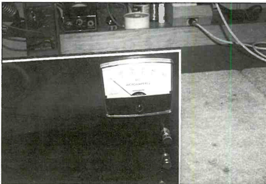
A 50- \mu A meter shows the relative signal strength of most audible stations. The meter is very useful for fine-tuning and finding the most sensitive tap positions.
