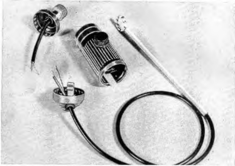
Probe ready for final assembly. Coax cable is wired in last.
