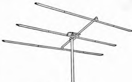
Fig. 3. Three-element yagi antenna. While shown here horizontally polarized, the elements may be oriented vertically in order to produce vertical polarization.
