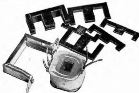
Coupling transformer T1 must be a miniature unit. If Argonne Type AR-162 is used, it can be reduced in size by removing the strap and laminations.
