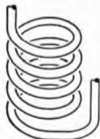
L2 4½" TURNS #12 WIRE, 3/4" LONG, 1/2" DIA.
