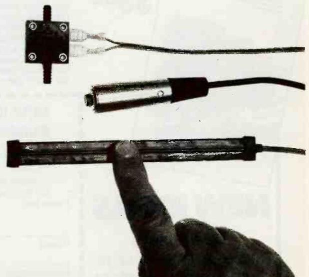
Some of the unusual switches that can be used with the Night Owl are the puff switch (top), cord switch (center), and the ribbon (or touch) switch (center).
