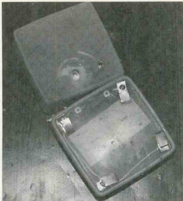
An ordinary plastic sandwich box—which can be found at drug and variety stores, or supermarkets—is used to house the series-connected batteries and components that make up the circuit.
