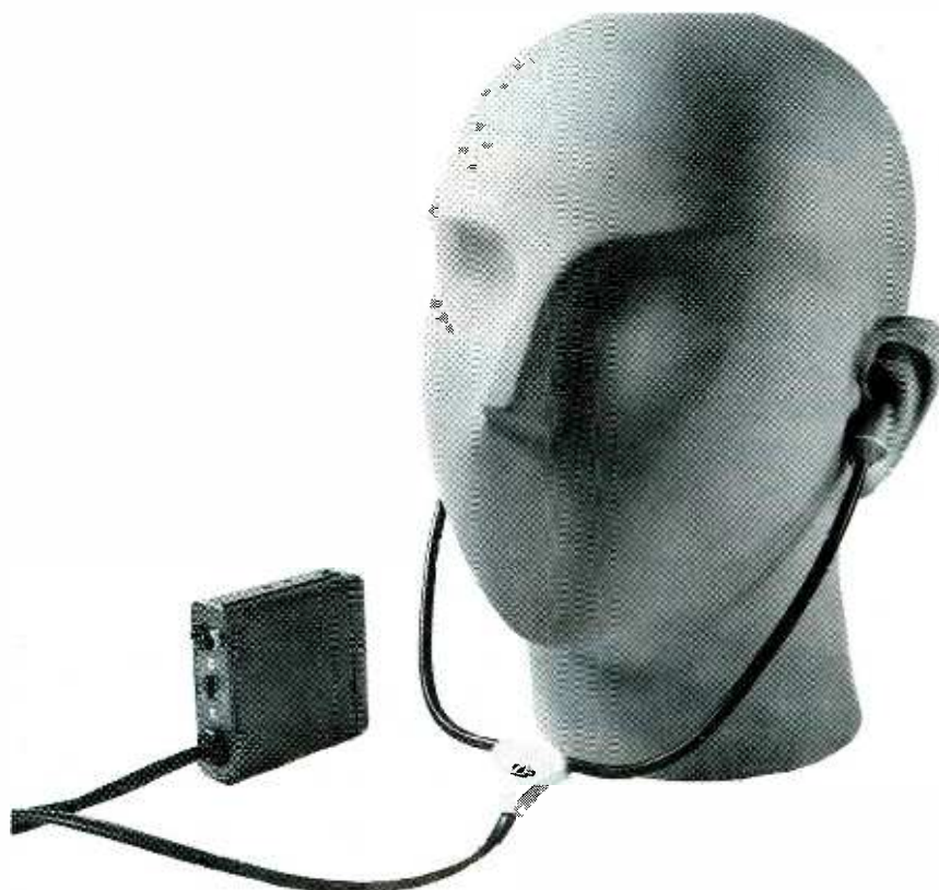
FIG. 1—IN TRUE BINAURAL RECORDING, a mechanical replica of the human head and ears ensures the proper capture of phase relationships. This is the MKE 2002 binaural dummy-head stereo-microphone setup from Sennheiser. To hear the special stereo effects, the recording must be listened to with high-quality headphones.
