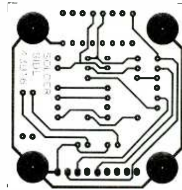
1 13/16 INCHES 2-DIGIT DISPLAY SOLDER SIDE.
