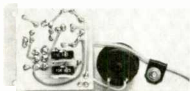
FIG. 2—THE SMALL PC BOARD can be secured to the front panel of the cabinet via S1's mounting nut. The board shown here is the author's prototype.
