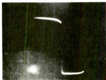
FIG. 4—THE ABOVE TRACE SHOWS the 60-Hz output from the inverter. Note that although the output is closer to a squarewave than a sine-wave, most of the high-frequency components have been removed.
