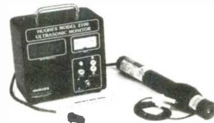
FIG. 5—LASERS HAVE many applications in industry. Here's a device that uses a laser to monitor the performance of an ultrasonic wire bonder, which is used in electronics production.
