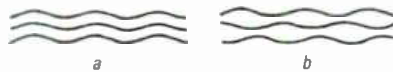
FIG. 3—IN LASER LIGHT, all of the waves are in phase; thus they are said to be coherent (a). In normal light, the waves have no phase relationship (b).
