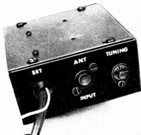
Fig. 3. Circuit must be built inside metal box to provide effective shield against r.f. interference that can be caused by ignition and other noises.
