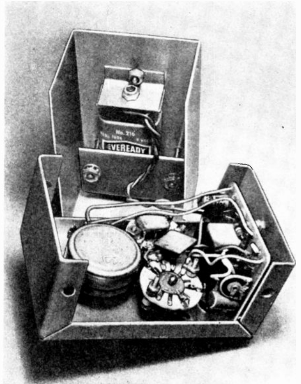
Fig. 4. In the author's unit, the battery is mounted on the rear cover so that, when the two sections are joined, it will not mechanically interfere with R2, S1, S2, or components mounted on printed board.
