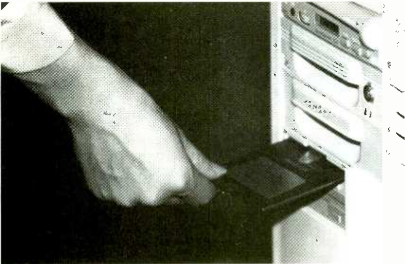
Fig. 2. Imation's SuperDrive packs 120MB of storage into a cartridge very similar to the familiar, ten-year old, 1.44MB diskette. An optical servo track allows the LS120 to achieve track density almost 20 times that of a 1.44MB diskette.
