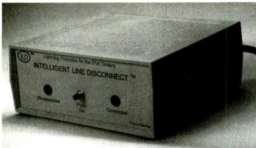
The Rabun Labs ILD is a protection system that automatically disconnects and grounds everything plugged into it when equipment is turned off; when the equipment is turned back on, all connections are restored. The simple "plug-and-play" unit, shown here, offers solid-state indicators, one-button operation, a "goof-proof" auto-disconnect timer, and filtering for power-line noise.
