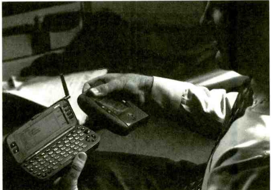
The Hewlett-Packard CapShare 910 is a hand-held scanner with built-in image preview, smart document assembly, and smart IR-based communications. Watch for it as a harbinger of a new breed of Information Appliance.
