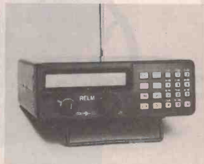
The Relm MS-180, which holds 100 memory channels, covers the 800-MHz band.
