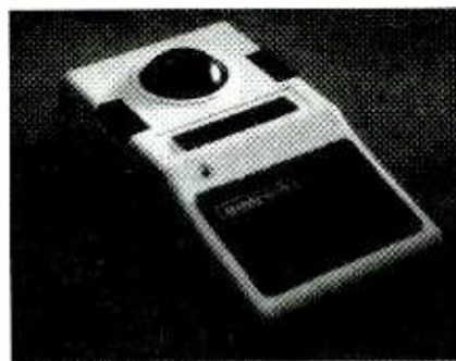
The Industrial Mouse-Trak is designed for harsh or controlled environments with a glass-filled Xenoy thermoplastic case and conformal coating on the PC board.
