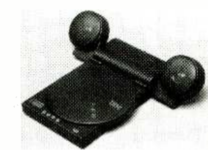
This portable CD-ROM drive from IBM has a fast PC-card interface to provide any notebook computer having a compatible slot with a CD-ROM drive, sound, and speakers.
