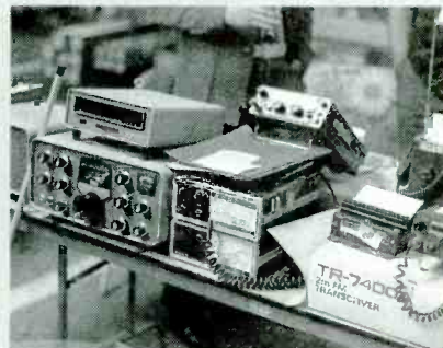
Though the firm quit making kits in the early 1990s, Heath's transmitters, transceivers, and receivers are still found at hamfests and swap meets. Take special care in purchasing used equipment built from kits, though; inspect the quality of the builder's assembly and soldering techniques before purchase.
