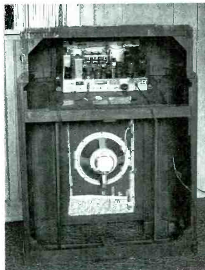
This is the complete rear view. The ten-inch speaker and huge magnet assembly below provide impressive sound indeed.
