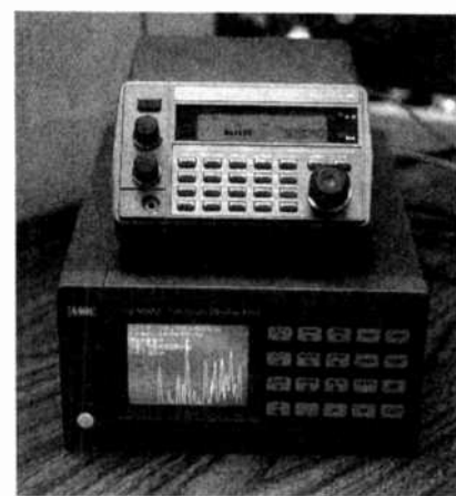
The AOR SDU-5000A Spectrum-Display Unit is shown here with its slave all-band receiver, the AOR-3000A. The combination provides excellent performance at an affordable price.
