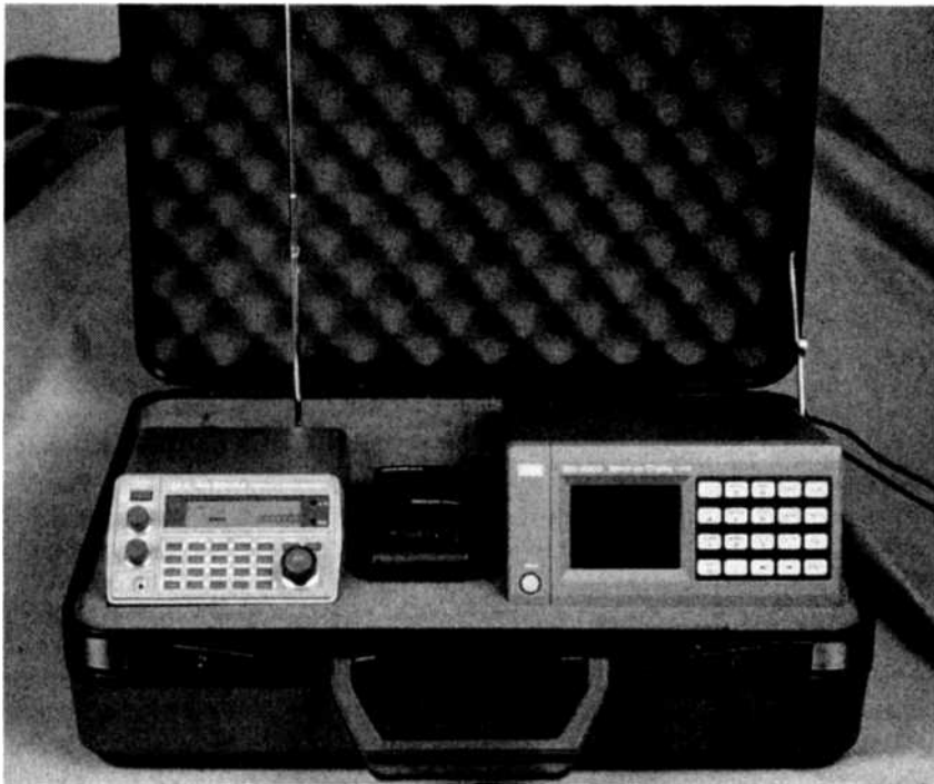
The two AOR units make a small operating package and could easily be used portably out of a large brief case.
