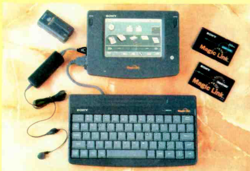
A number of accessories are available for the Magic Link personal communicator. Pictured here, counter clockwise from top left are a lithium-ion battery, telephone headset, data-entry keyboard, memory card, and pager card.
