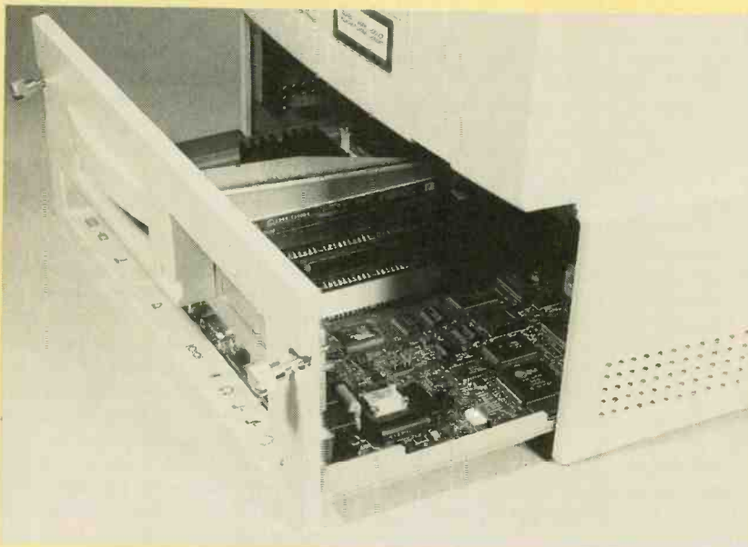
The Presario's motherboard contains many of the functions that would normally be incorporated on separate plug-in cards. For upgrades, the motherboard simply slides out in a drawer from the main chassis. Note the clearly labelled input and output jacks.
