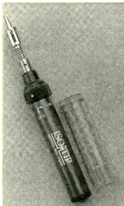
This Wahl butane-powered soldering iron and torch is for heavy-duty electrical jobs—not for delicate PC-board work. Ideal for hobbyists and technicians, especially in outdoor applications, the cordless and refillable iron features an aluminum body and even-flow valve for a uniform flame. (Photo courtesy Wahl Clipper Corporation.)
