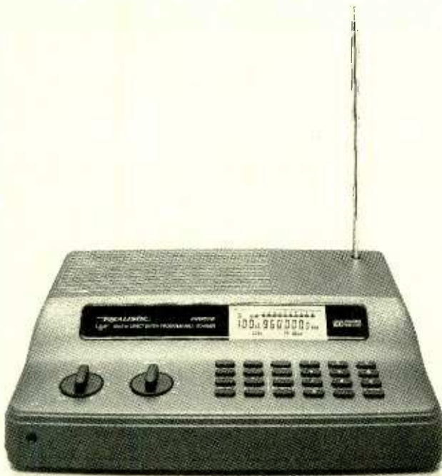
The Radio Shack PRO-2027 desktop scanner offers "Hyperscan" rapid scanning.
