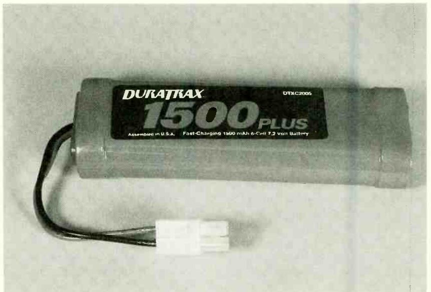
This rechargeable Ni-Cd pack has 6 cells. You can purchase 7-cell packs for even more punch.
