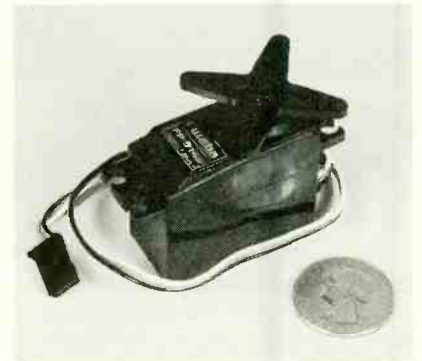
In addition to a decoder chip, a servo contains a motor, gearbox, and output shaft. The servo can hold or adjust the position of its output shaft based on the signal from the transmitter.
