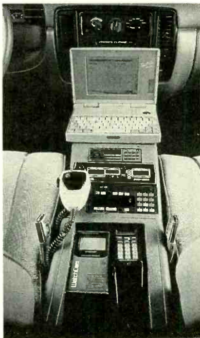
The center console in a Cruiser holds a laptop computer, a closed-circuit monitor, a cellular phone, a two-way radio, and more high-tech electronics.
