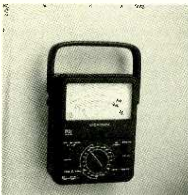
This Micronta 10-megohm, FET-input multimeter operates like a solid-state VTVM, letting you troubleshoot and test sensitive circuits with minimal loading. It also has a jumbo 5-inch, tri-color scale. (Photo courtesy Radio Shack)
