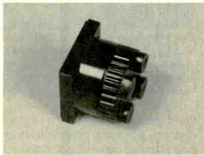
This tiny sound element makes a beeping noise when current flows in one direction and a warbling sound when the current is reversed. It will also change sounds if you twist its top 180°.
