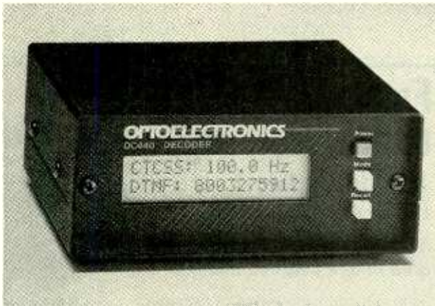
The Optoelectronics DC440 can read CTCSS tones, digital codes, and DTMF (Touch-Tone) characters simultaneously.
