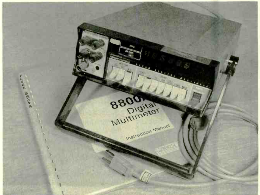
The Fluke 8800A was a great buy at $295 from Naptech. Its 5½-digit readout can resolve microvolts and milliohms. It came with a manual and a 6-month warranty.
