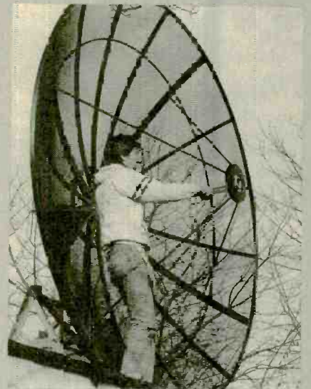
Here, the focal length is being checked for accuracy.
