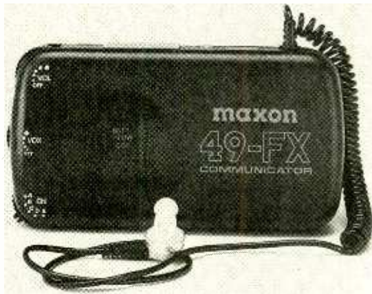
This Maxon 49-FX five-channel transceiver operates in the 49.82–49.90-MHz band. Have you ever monitored there?
