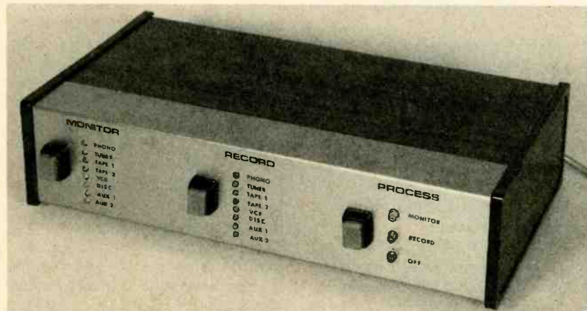
The author's prototype incorporated two audio-switcher circuit boards and a switching network.
