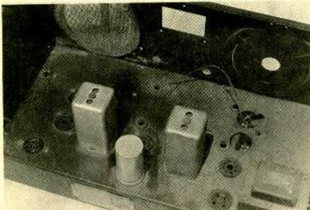
The partially cleaned main chassis. The area shown at the left has been washed and wiped; the area at the right is still "as found."
