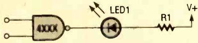
Fig. 6. A CMOS-based gate can sink current much like a TTL gate in order to activate an LED.
