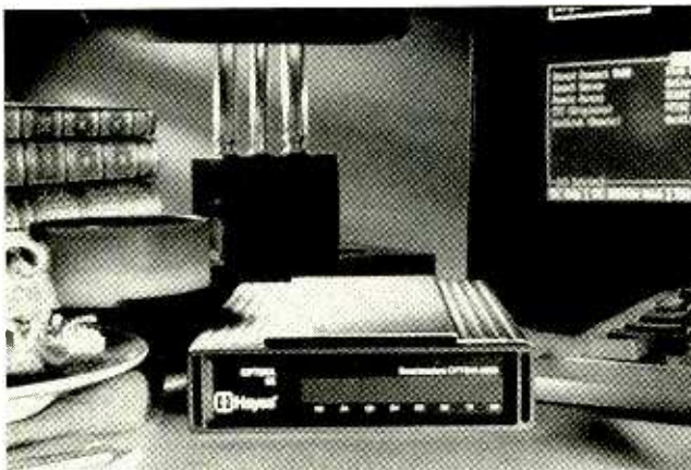
Hayes' Optima 96 is a V.32/V.42bis modem that's blazing new trails in price (about $450) and performance.
