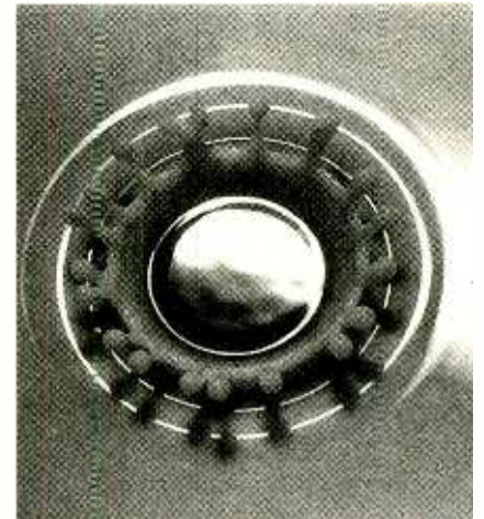
This milk crown—a drop of milk actually splashing off a solid surface—is but one example of an action that requires split-second timing to capture on film.
