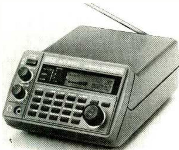
With a scanning range of 100 kHz to 2036 MHz, and an optional frequency-logging and -analysis system, AOR's model AR3000 is truly a state-of-the-art scanner.
