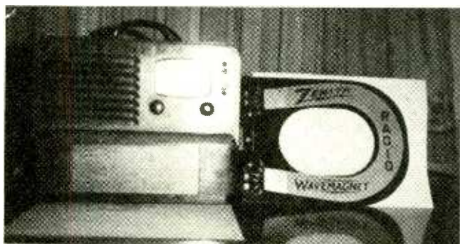
Kent A. Ponton sent along this shot of his latest garage-sale find, a wood-cabinet Zenith portable (model T197604), complete with wavemagnet antenna.
