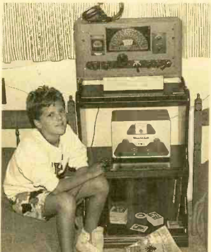
Brady McGhee, KA9VDE can work the world from his bedroom with a Heath DX-40 and RME-45. The RME was typical of the better receivers built after the war but used a mechanical bandspread system.
