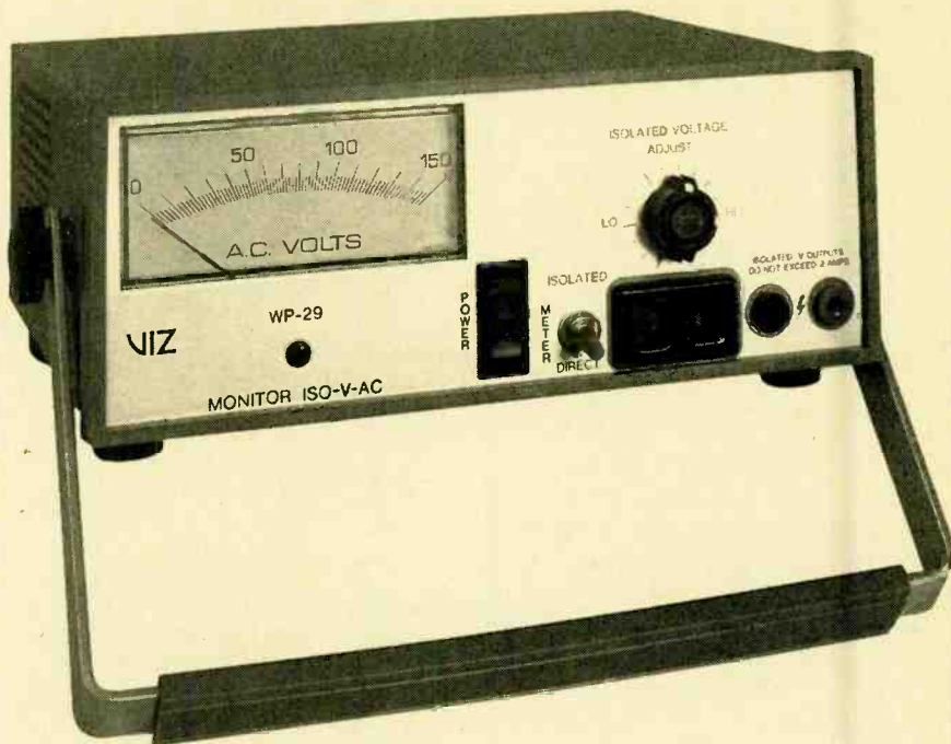
Some isolation transformers, like the unit shown here, allow you to vary the amount of voltage delivered to a device. That feature is very useful in troubleshooting faulty gear.
