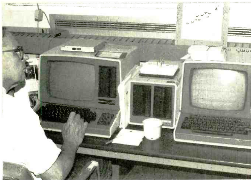
Fig. 3. Practice text for WIAW code-practice transmissions are taken from the text of league publications, and is entered into a Heath H-89 computer that, in turn, controls the WIAW transmitters.
