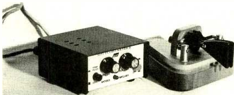
The MFJ-401 Electronic Keyer (from MFJ Enterprises) and a Vibroplex key. The Vibroplex key—essentially a paddle-operated single-pole double-throw switch—is especially designed for use with electronic keyers. The MFJ-401 keyer offers speed control, and the ability to effect a contact closure on dash in order to simulate a bug and to tune-up transmitters.
