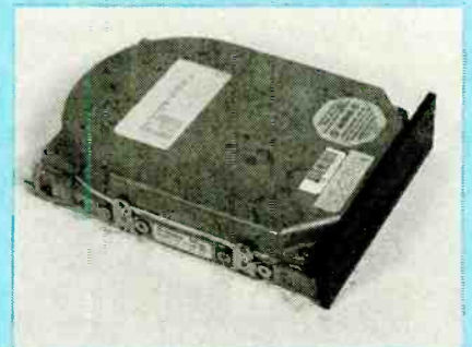
Half-height hard-disk drives designed to fit into one of the slots intended for floppy disk drives, can give you super storage in a very tiny space. Technology has really changed!
