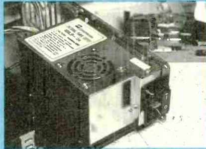
This is a 150-watt replacement power supply for the PC/XT installed in a PC/XT cabinet. The number of screws to mount your power supply will depend on your cabinet.
