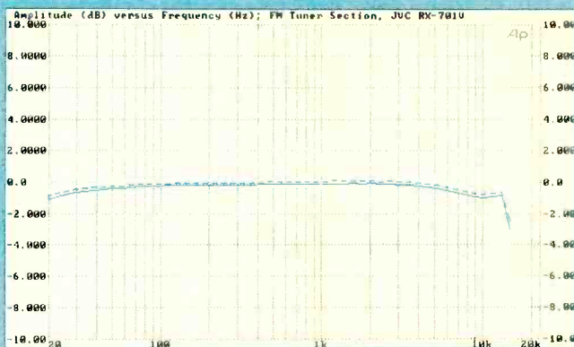
The frequency response was virtually flat over the entire FM audio range.
