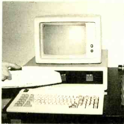
Vacuum all the small air vents of the computer and disk drive openings, as well as any other openings in the case where air can enter.
