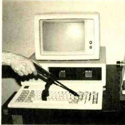
Using a small soft attachment, clean the keyboard with a small hand vacuum.
