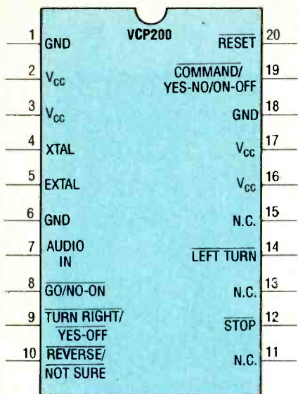
Fig. 1. This pinout diagram will prove invaluable if you choose to wire your Voice-Operated Switch on perfboard as the author did in building his prototype.
