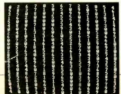
Fig. 9. Random digits generated by a program controlled by a radiation meter.
