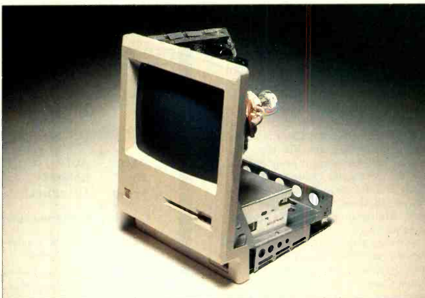
Built-in monitor and 3.5" disk drive.
