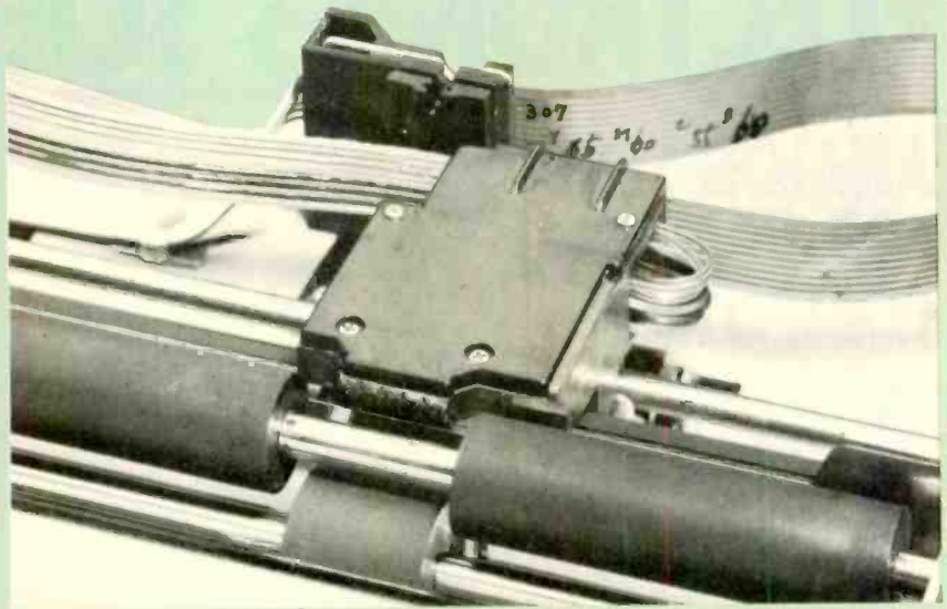
A horizontal array of four ink nozzles moves across the paper.
