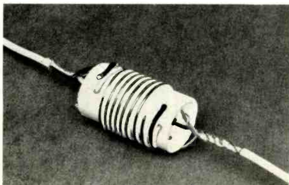
Fig. 7. A completed trap ready to be soldered. Note that the Rainbow Wire has been closely wound around the form.
