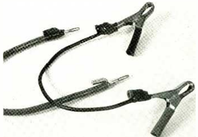
Fig. 4. Shunts can be terminated in banana plugs or small clips as shown here.
