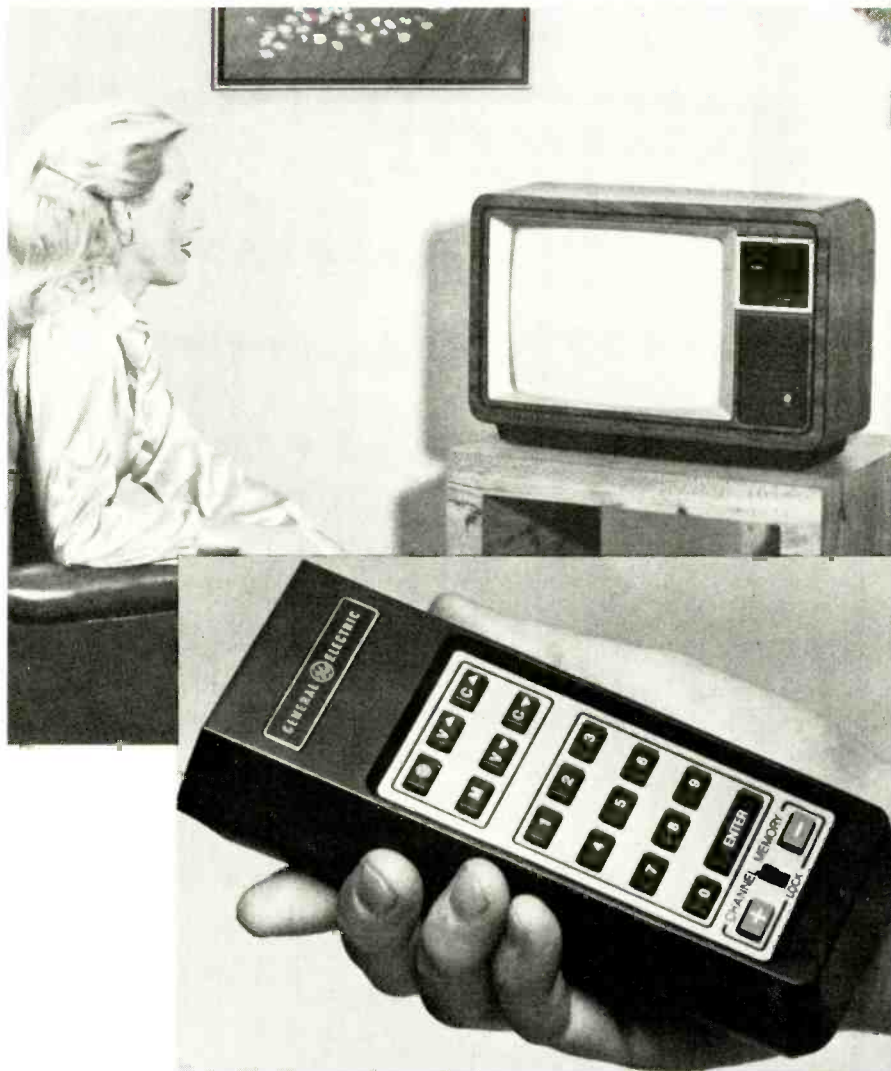
Fig. 1. The remote-control system (the Transmitter is shown here in the inset) is versatile and quiet. It operates on an infrared beam and controls 82 channels.
