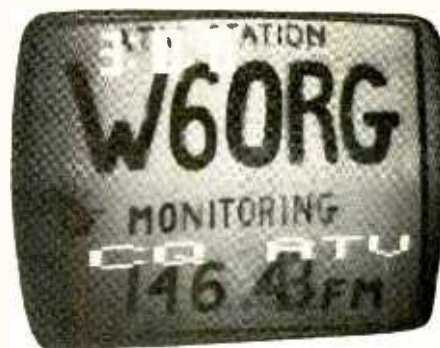
Off-the-air ATV picture as transmitted by amateur Tom O'Hara, W6ORG. Note superimposed clock and CO ATV. Highly directional beams and two-meter talkback circuits are usually used.
