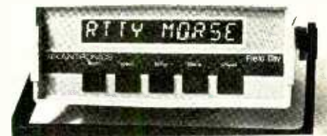
Kartronics Morse-code radioteletype reader.
