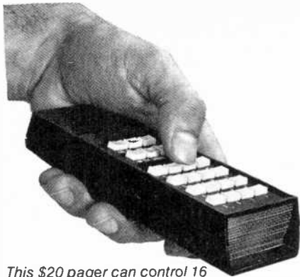
This $20 pager can control 16 of either your appliances or your lights. There's no installation required and the complete story is explained below.
